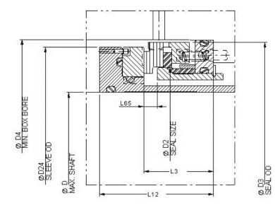
The 8628VSC secondary containment seal is sized on known equipment dimensions used in pipeline applications. Sizes to fit common pipeline pumps up to 6.500 inch shafts.
