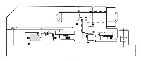
The dry tandem arrangement uses the high duty version of the SBOP backup seal to provide operational security without the expense of a liquid buffer system. In the event of failure of the inner seal, the SBOP will prevent loss of the pumped fluid to the atmosphere. This can be detected by use of a pressure switch.
