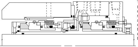
The dual, unpressurized (tandem) arrangement consists of two seals in series. The inner seal operates on pumped fluid and the outer seal normally operates on a low pressure buffer liquid. The outer seal is designed to provide a full-duty backup service.
