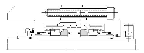
This dual pressurized (double) arrangement consists of two seals face to face and operating on a barrier liquid. Any leakage from the inner seal will be of barrier fluid into the pumped product. The inner seal includes a double balance line for reverse pressure protection.
